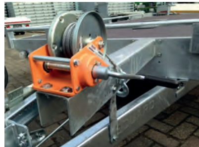
Fig. Winch The cable winch T1-208
